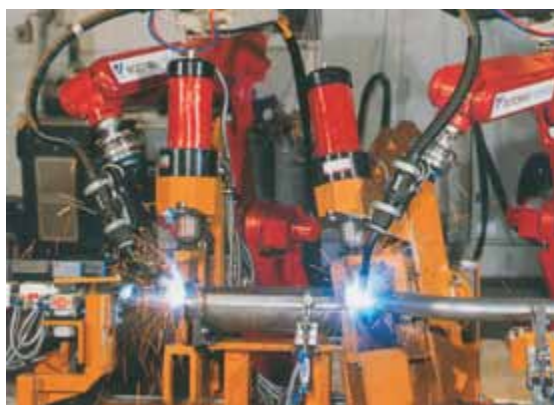
Welding fixture for exhaust components
