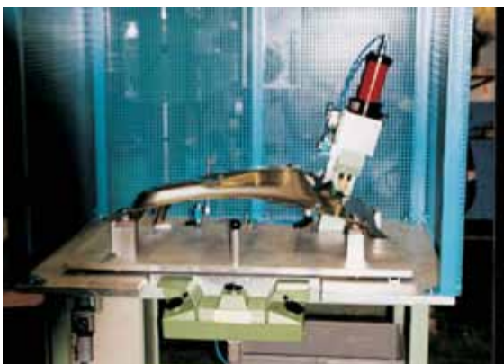
Device for holes Ø 8 in sheet metal
